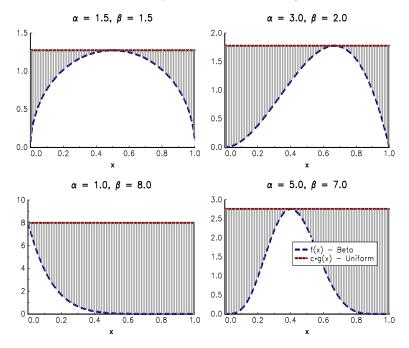
FIGURE 13.3: Rejection sampling applied to the beta distribution
